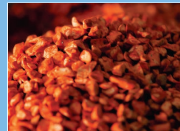
The BASF-N 2 O decomposition catalyst converts nitrous oxide into harmless nitrogen and oxygen.
