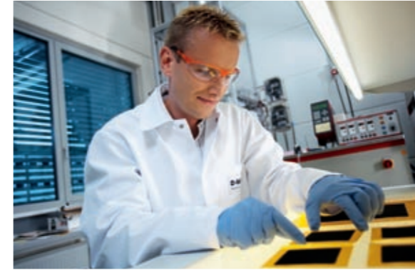
Manufacture of membrane electrode assemblies (MEAs). The MEA is the heart of the fuel cell.
